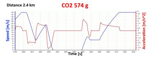
Figure 8: Single vehicle speed profile, with accident
