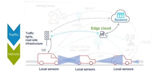
Figure 14: Implementation options with V2I (I2V) communication.
