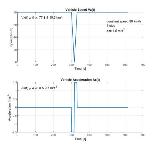
Figure 11: Synthetic speed profile for a constant approaching speed of 80 km/h used for the impact estimation for avoiding stops at intersections.
