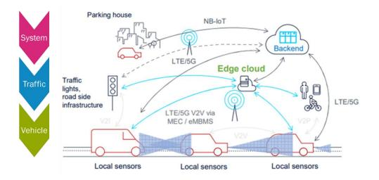
Figure 15: Implementation options with V2N (N2V), V2N2I (I2N2V), and V2N2V communication.
