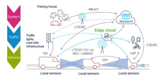
Figure 16: Implementation option with hybrid infrastructure including a combination of different communication types, e.g., V2V, V2I (I2V), V2N (N2V), V2N2I (I2N2V), V2N2V.
