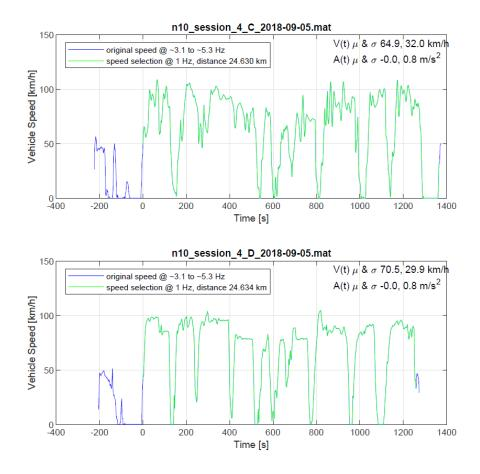
Figure 7: Comparison of speed profiles with ACC (upper figure) and CACC (lower figure).
