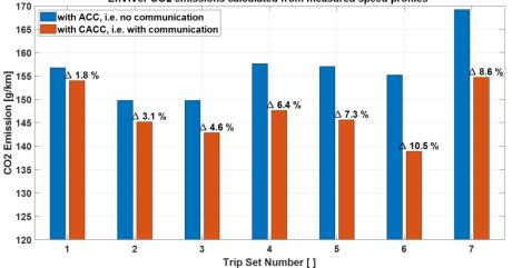
Passenger cars with ACC or CACC on Dutch 2x2 lane rural road with controlled intersections (100-80-50 km/h) EnViVer CO2 emissions calculated from measured speed profiles
