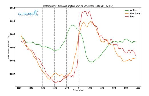
Figure 10: Average fuel consumption profiles for crossing the intersection with or without stop (No Stop/Slow Down/Stop).
