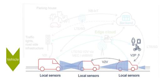
Figure 13: Implementation options with V2V communication.
