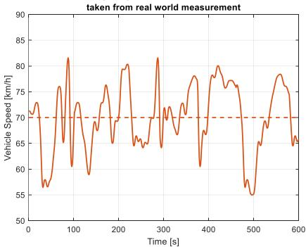
Simulated speed profile for 80 km/h road, variations taken from real world measurement
