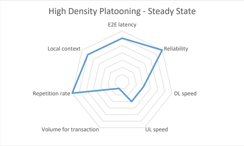
Figure 28 Spider Diagram – ‘High-Density Platooning Host Vehicle to Cloud Use case HV-CA’
