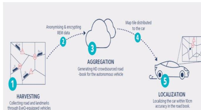
**Figure 45 Mobileye HD Mapping Process**
