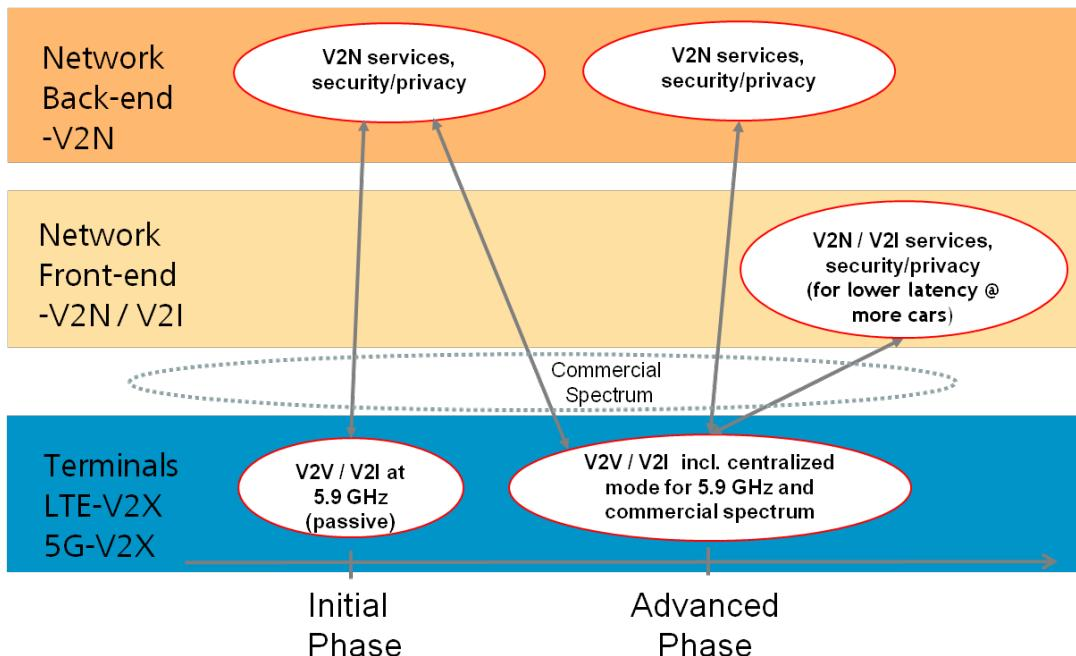
It is important to highlight that V2V and V2I safety services over ITS spectrum are offered for no V2X service fees, so a primary difference between 802.11p and C-V2X would be improved performance with C-V2X. This functional and deployment architecture allows for multiple business models, another difference between 802.11p and C-V2X.
