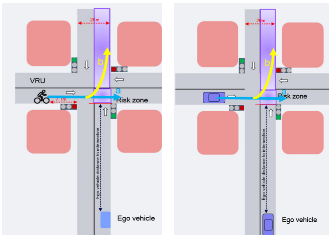
Figure 2 Scenario 1 (1a and 1b) with VRU approaching from left Figure 3 Scenario 2 (2a and 2b) with vehicle approaching from left
