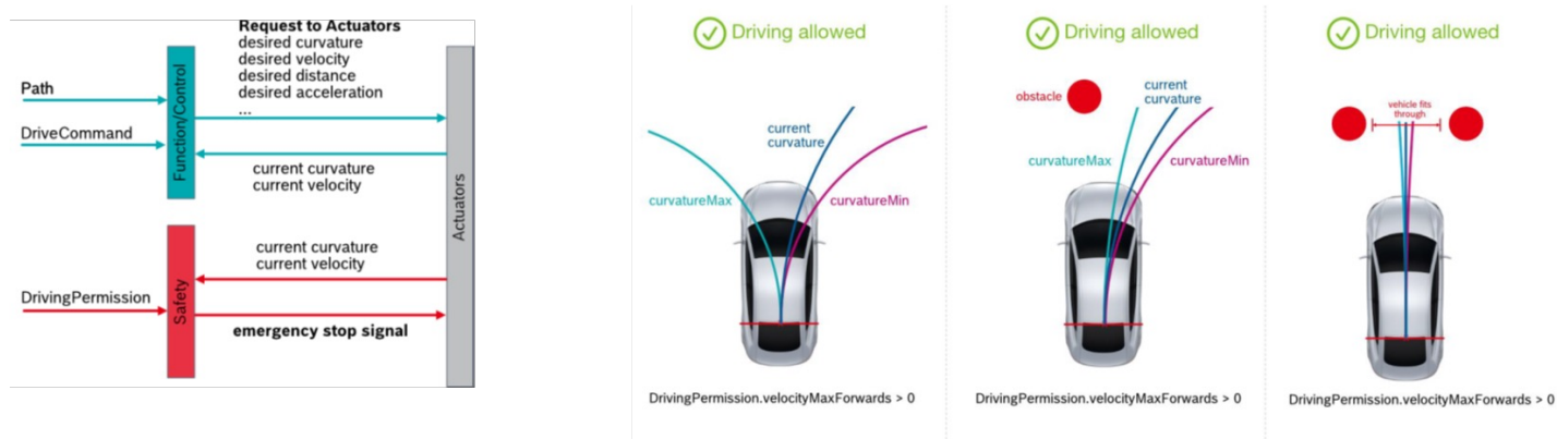
Figure 5 – Group Start safety concept (assumed to be same in general as AVP)
