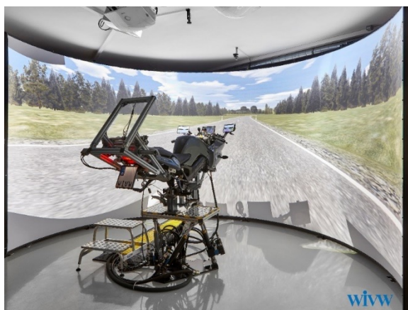
Figure 98: DESMORI Dynamic motorcycle riding simulator at WIVW
