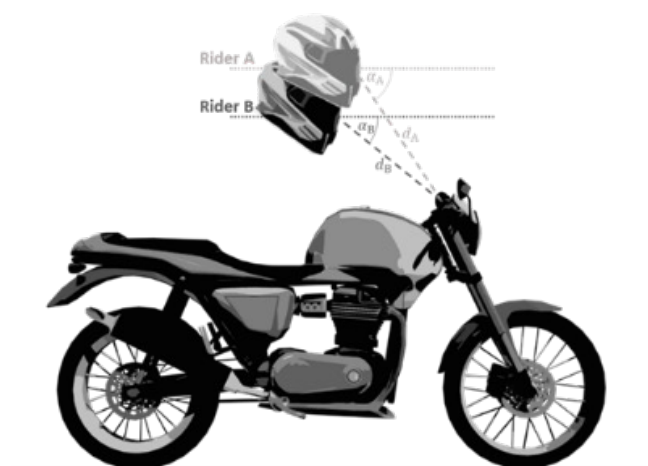
Figure 101: Schematic representation of different dashboard downward angles as a function of different rider heights
