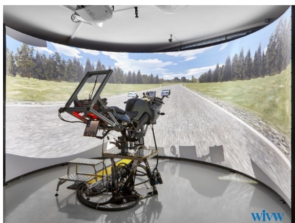
Figure 98: DESMORI Dynamic motorcycle riding simulator at WIVW
