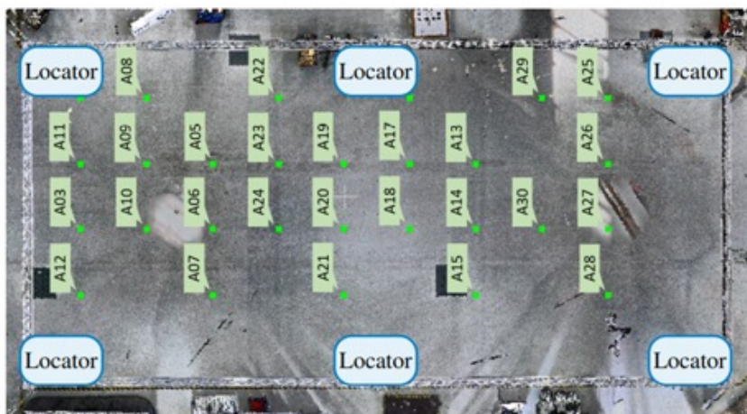
Figure 21: Ground truth position of the UE on the shop floor [26]
