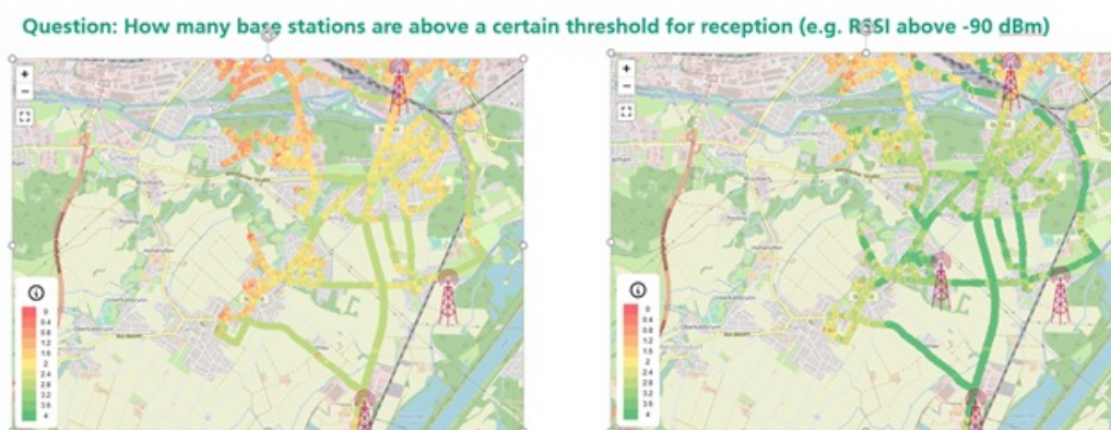
Figure 32: Example simulations with three and four GnodeBs
