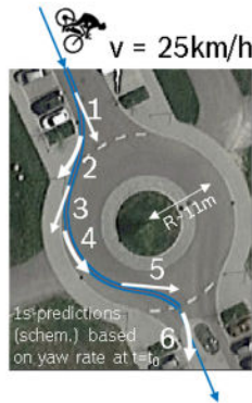
Figure 12: Example of path prediction based on heading, speed, acceleration and curvature
