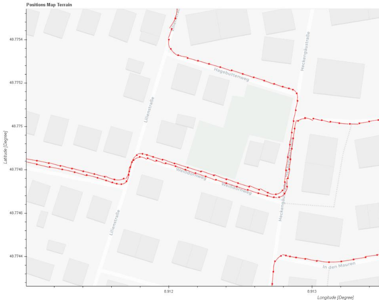
Figure 21: Bicyclist's path prediction based on bike sensors (inertia sensors and more) and bike models (dots: real positions; lines: predicted path)
