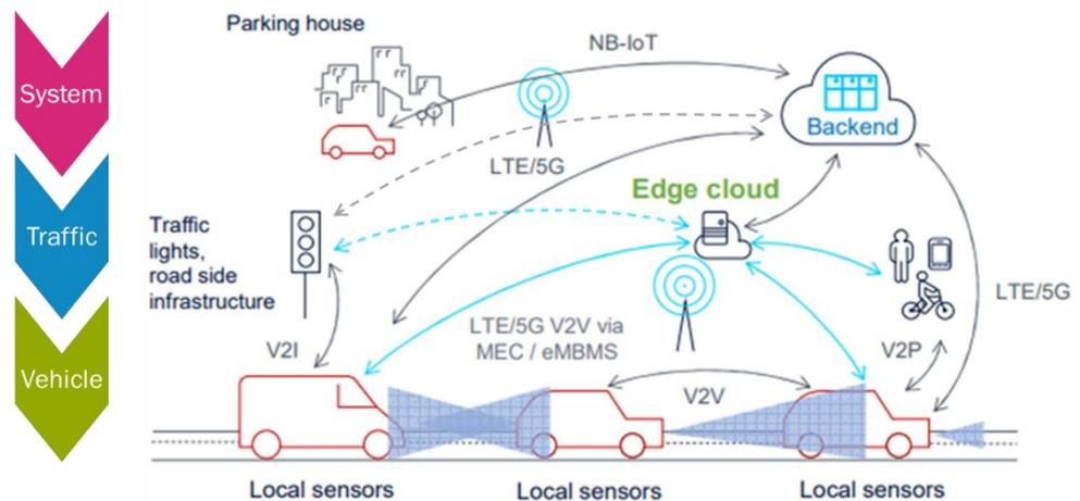
Figure 16: Implementation option with hybrid infrastructure including a combination of different communication types, e.g., V2V, V2I (I2V), V2N (N2V), V2N2I (I2N2V), V2N2V.
