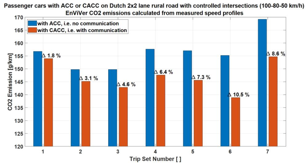
Figure 6: Emission reduction per trip, CACC compared with ACC on a 2x2 lane rural road with controlled intersections.
