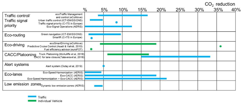
Figure 17: Impacts of different applications classified per level on which the impact is described.
