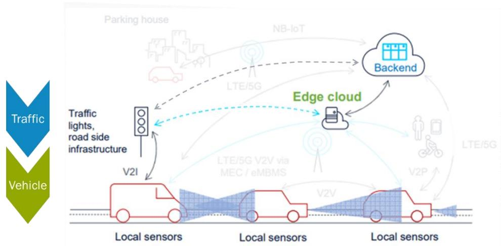
Figure 14: Implementation options with V2I (I2V) communication.
