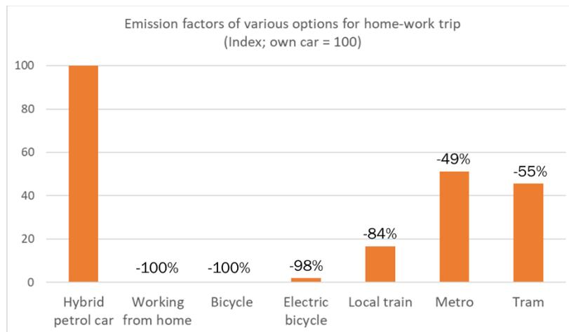
Figure 4: Emission factors of various options for home-work trip, as compared to the emission factor of hybrid cars (emission factors for the Netherlands, source of emission factors for different modes: <https://www.co2emissiefactoren.nl/lijs-emissiefactoren/>)
