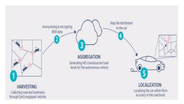
Figure 45 Mobileye HD Mapping Process
