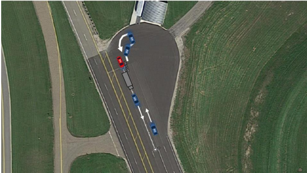
Figure 47: Map of the North Circle at FPG Road A Showing NLOS Non-Intersection Test Setup
