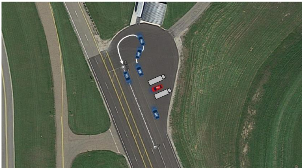
Figure 54: NLOS Test Setup for the Approach from the Left
